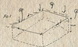
fig. 1. Dig a pit about 700mm deep. It should be long and wide enough to fit all the food but not too much gaps. 1 meter x 1.5 meter is a good starting point.
